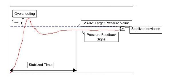
Figure 4.4.103 Diagram of pressure feedback value
