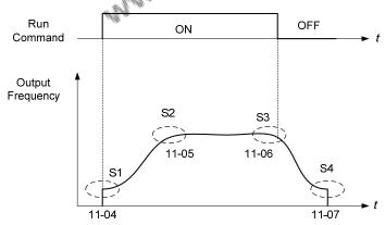
Figure 4.4.76 S curve characteristic
