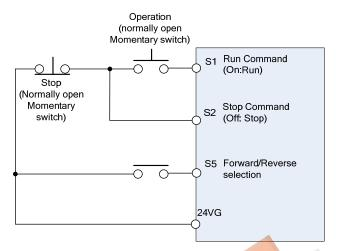
Figure 4.4.2 Wiring example of 3-wire
