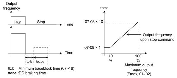
Figure 4.4.50 DC braking to stop
