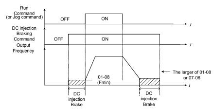
Figure 4.4.21 DC braking timing diagram
