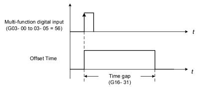
Figure 4.4.88 Operation of offset time
