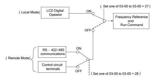
Figure 4.4.20 Remote mode operation selection
