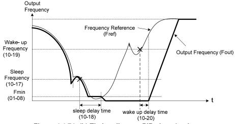
Figure 4.4.74: (b) Timing diagram PID sleep / wakeup
