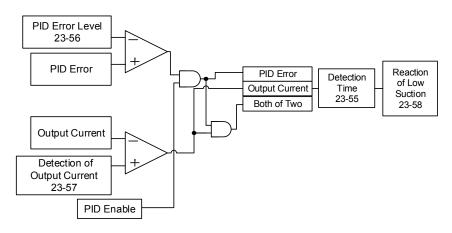
Figure 4.4.115 Diagram for the process of low suction
