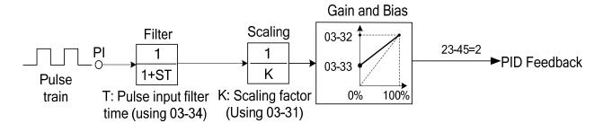
Figure 4.4.24 Pulse input adjustment
