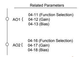
Figure 4.4.40 Analog outputs and related parameters
