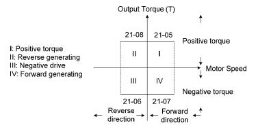
Figure 4.4.101 Torque limit setting
