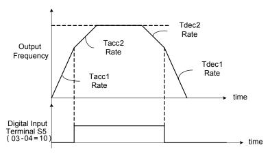
Figure 4.4.6: Terminal S5 switch between Tacc1/Tacc2 and Tdec1/Tdec2
