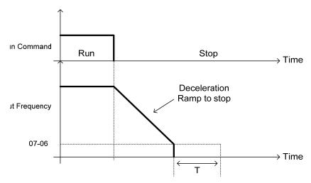
T: DC Braking Time at stop (07-08)
