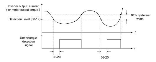
Figure 4.4.64 Low torque detection operation
