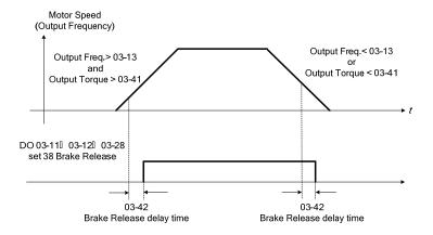
It is also recommended to be with the use of start and stop frequency locked function (11-43~11-46), shown as the following figure:
