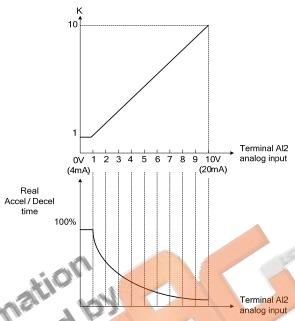
Figure 4.4.33 Acceleration / deceleration time reduction coefficient
