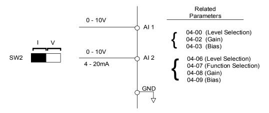
Figure 4.4.25 Analog inputs and related parameters
