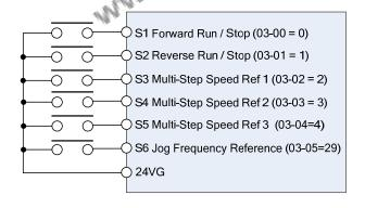
Figure 4.4.14 Control Terminal Wiring Example
