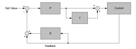
Figure 4.4.69 PID control for feedback differential value
