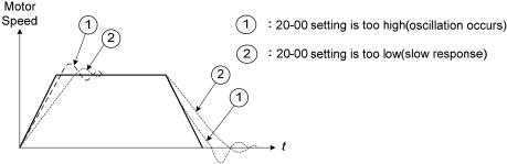
Figure 4.4.97 System response of ASR proportion gain
