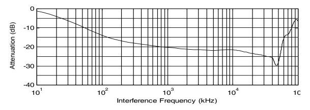
Figure 11.3.1 Frequency attenuation characteristics (10 windings case)
