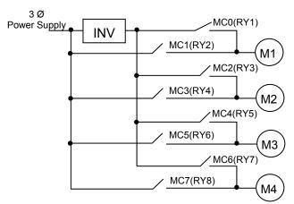
Figure 4.4.117 Cycle modes of inverter pump
