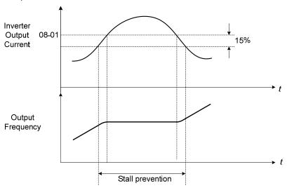
Figure 4.4.57 Stall prevention during acceleration
