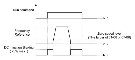
Figure 4.4.84 Zero-speed braking operation
