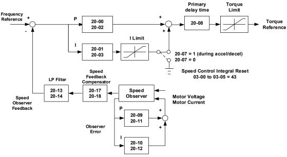
Figure 4.4.95 ASR block diagram (SLV mode)
