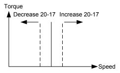
Figure 4.4.99 Effect on the torque-speed curve from 20-17
