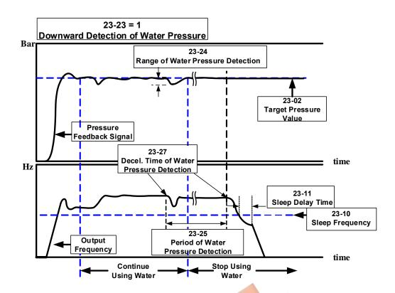
Figure 4.4.110 Diagram for downward detection of water pressure
