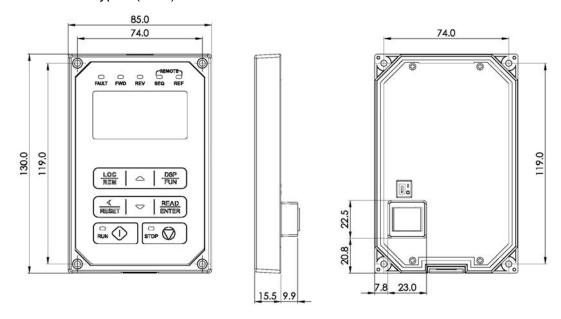
Figure 11.5.3 Dimensions of LCD keypad (IP55)
