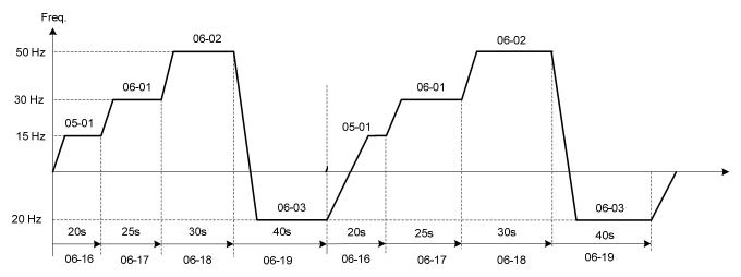
Figure 4.4.43 Periodic automatic operation
