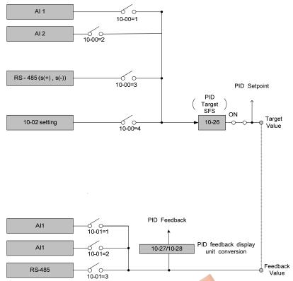
Figure 4.4.71 PID input selection
