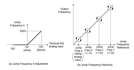
Figure 4.4.38 Jump frequency 4 setting operation
