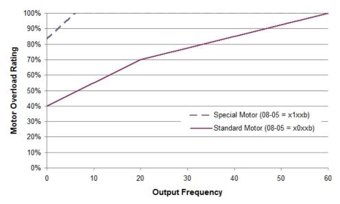
Figure 4.4.62 Motor overload rating at different output frequencies
