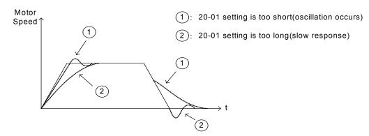
Figure 4.4.98 The response of ASR integral time
