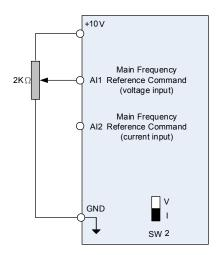
Figure 4.4.4 Analog input as main frequency reference command
