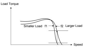
Figure 4.4.90 Slip compensation output frequency
