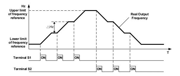
Mode3: When 03-39 is not set to 0Hz and terminal conduction time is larger than 2 sec, frequency variation depends on acceleration/ deceleration.
