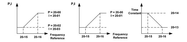
Figure 4.4.96 ASR gain setting (SLV mode)
