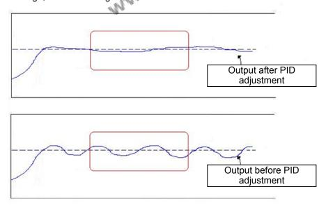
Figure 4.4.104 Diagram for PID parameter adjustment
