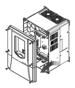
**Step 5:** Check the inside waterproof gasket is not pulled away from cover while opening the cover
