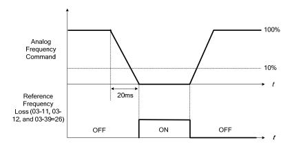
Figure 4.4.81 Operation for reference frequency loss
