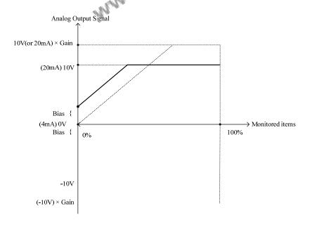
Figure 4.4.41 Analog output level adjustment
