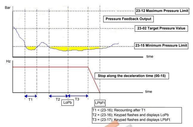
Figure 4.4.108 Diagram for warning to stop under the limit of low pressure
