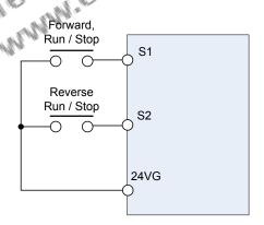
Figure 4.4.1 Wiring example of 2-wire
