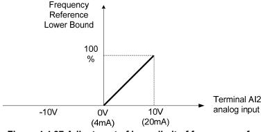
Figure 4.4.37 Adjustment of lower limit of frequency reference
