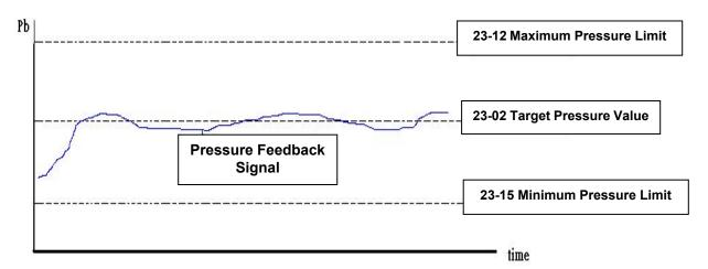
Figure 4.4.106 Diagram for pressure feedback limit
