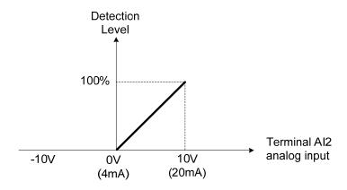
Figure 4.4.35 Over-torque/less torque detection level adjustment
