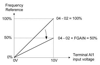
Figure 4.4.29 Frequency reference gain adjustment (example)
